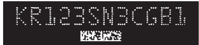
In-Sight wafer readers reliably read a wide array of marks, including the SEMI M1.15 300mm wafer mark shown above.
